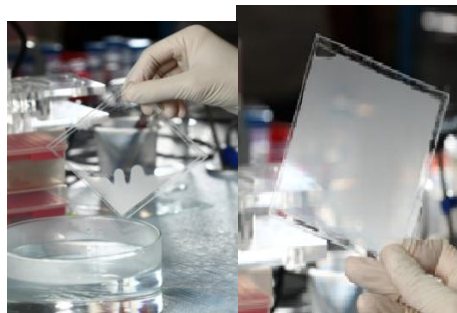
Glass with smart materials new chemical composition responds quickly to external heat and changes from transparent to translucent
